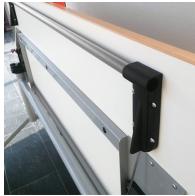
Triggering of the folding function by means of 2-hand safety operation
